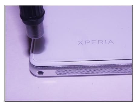
Heat along the edges of the back cover using a heat gun to soften the glue.
