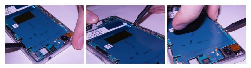
Carefully pry up on the four sides of the motherboard using the plastic spudger til it separates from the base of the phone.
