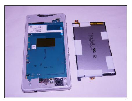
Remove the battery from the device
