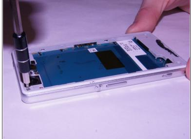
• Unscrew the four screws on the corners of the back frame using the JIS #00 screwdriver.
