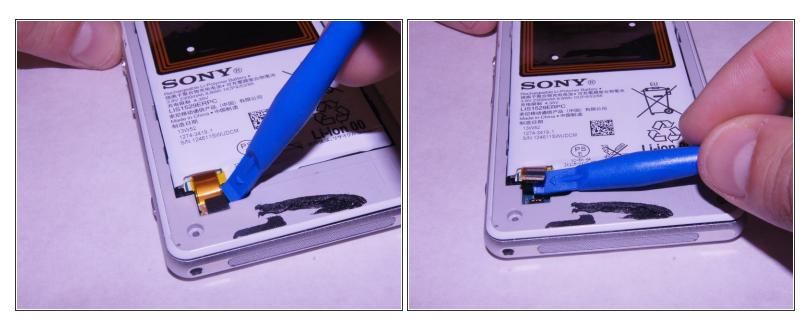
• Carefully disconnect the battery from the logic board by using the plastic spudger as a lever.
