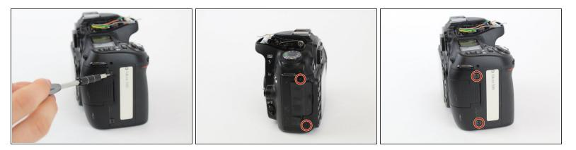
Using a Philips #00 screwdriver, remove the four 6.2mm from the left and right sides of the outer cover.
