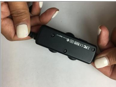
Flip the audio jack casing so the screws are facing you.
