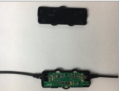
Insert a plastic opening tool between the two plastic pieces to pry it open.
