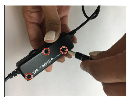
Remove the three 1.1 mm screws using a Phillips #00 screwdriver.
