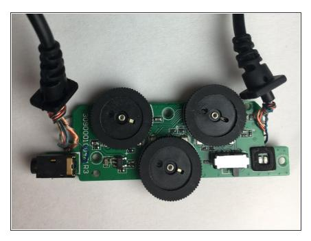
Carefully remove the audio board from casing.
