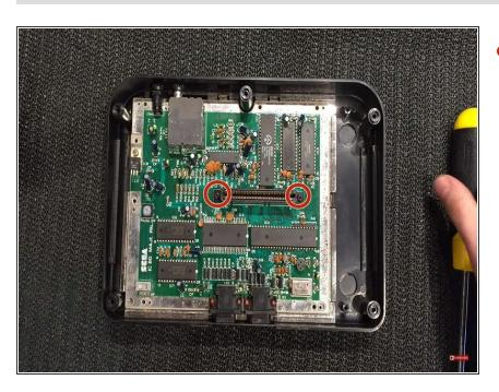
Remove the 2 screws thats holding the cartridge slot down
