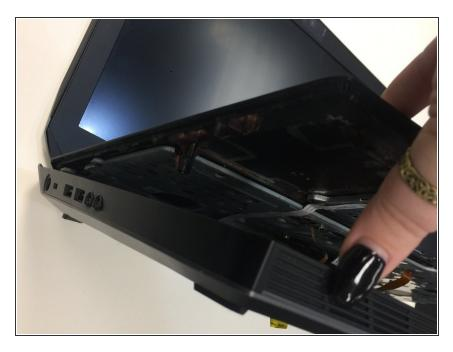
• Gently, separate and remove the plastic palm rest.
