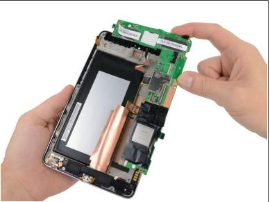
Carefully lift the motherboard assembly out of the Nexus 7, minding any cables that may get caught.
