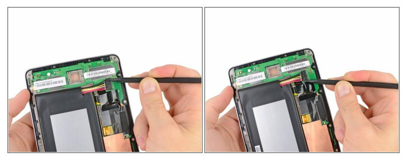
• Using the tip of a spudger, push first on one side then the other to "walk" the battery cable straight out of its socket on the motherboard.
