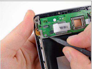
Use the tip of a spudger to remove the warranty seal stickers.
