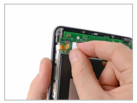
Peel back the label covering the power and volume button ZIF connector.
