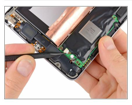
Using the tip of a spudger, push the speaker cable straight out of its socket on the motherboard.
