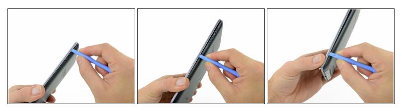
Insert the plastic opening tool between the rear panel and the front panel assembly near the power button and pry up at several points along the right edge of the Nexus 7.
