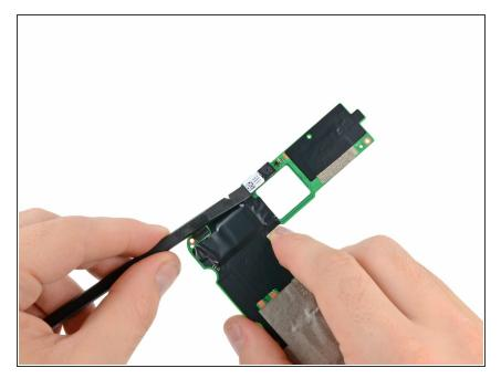
Use the flat end of a spudger to pry the front-facing camera straight up off its socket on the motherboard.
