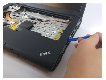
Snap off the top cover with a plastic opening tool, ensuring that the tabs don't snap back on.
