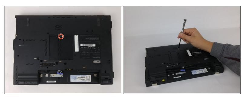
Loosen (do not remove) the 14.0mm screw in the DIMM slot cover with a Phillips #2 screwdriver.
