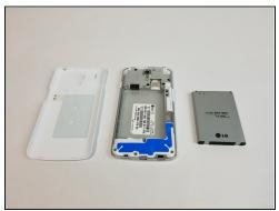
With your finger, pry the battery out through the crease made for removal.
