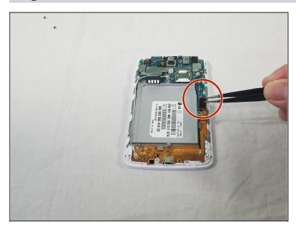
Using the precision <u>tweezers</u> set lift the copper tab located on the right side of the device.
