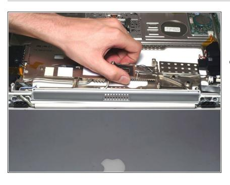
Grasp the metal heat exchanger and pull up and away from you. You may need to move the inverter cable on the right side of the computer in order to rotate the heat exchanger.
