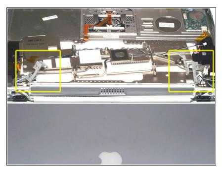
Lift up the metal brackets on either side of the upper case.
