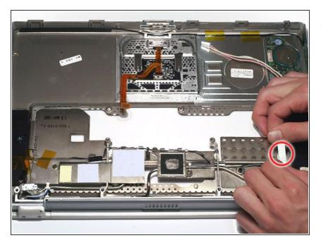
Disconnect and remove the pink and white inverter cable, removing tape as necessary.
