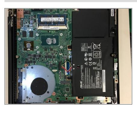
the battery must be removed so there is no power running to the disk drive. Follow the battery replacement guide <u>here.</u>
