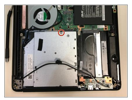
Unscrew the one screw on the disk drive with a Philips head screw driver 1.
