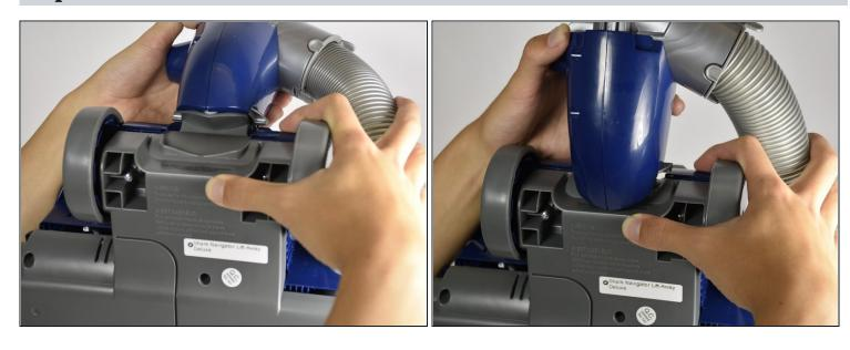
• Move the blue fulcrum connecting the bottom and the main body of the vacuum cleaner back and forth to loosen up crevice between the two halves of the roller brush enclosure.
