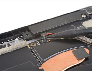
Use the point of a spudger to lift the right speaker connector up and out of its socket on the motherboard.
