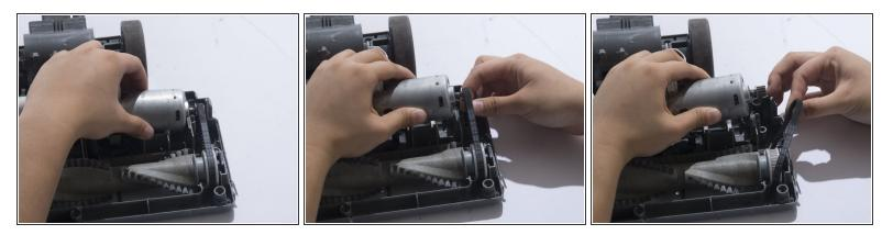
• Remove the belt from the motor gear by sliding the belt to the right.
