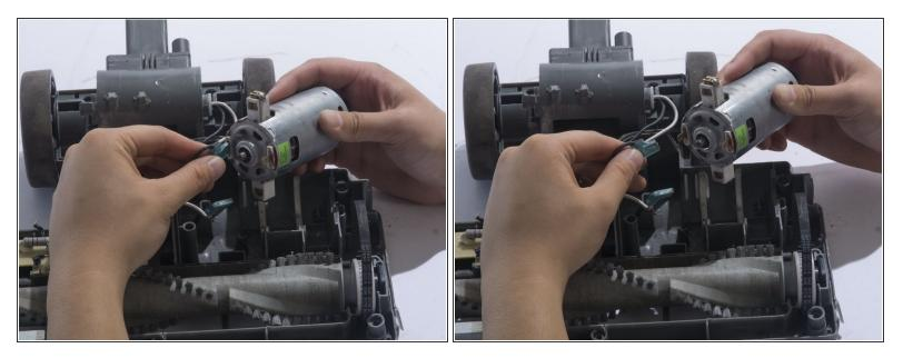
• Remove the black metal wire connector from the motor.
