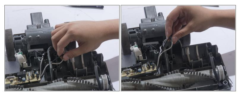
• Free the black and white cables that were previously attached to the motor from their slot.
