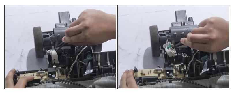
• Lift up the wire housing from the plastic base using tweezers.
