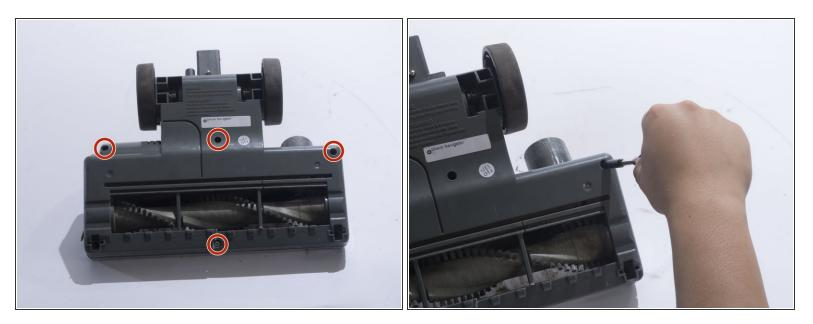
Remove the four 18mm screws located on the top corners and the bottom/middle of the vacuum head using a JIS 1 screwdriver.
