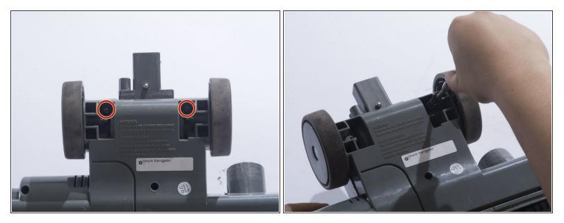
• Remove the two 18mm screws located on the inside of the large wheels using a JIS 1 screwdriver.
