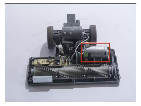
• Locate the motor on the top right corner of the vacuum head shell.
