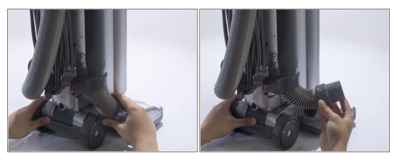
• Detach the hose connected on the bottom of the vacuum by pulling it out of the casing.
