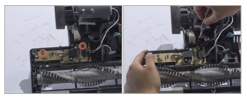
• Remove the two 12mm screws using a JIS 1 screwdriver.
