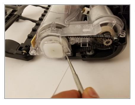
Pry tab out with a flat head screwdriver or any wedge-like tool.
