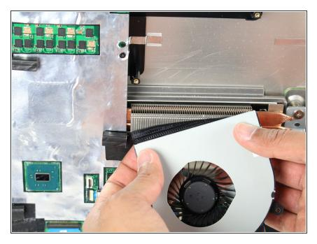
Remove the fan by peeling off the black electrical tape holding it against the heat sink vents.
