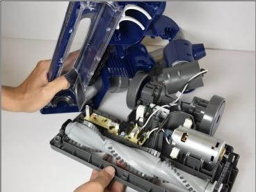
• Lift the grey frame off the bottom of the vacuum cleaner with your hands and place it on a flat surface.
