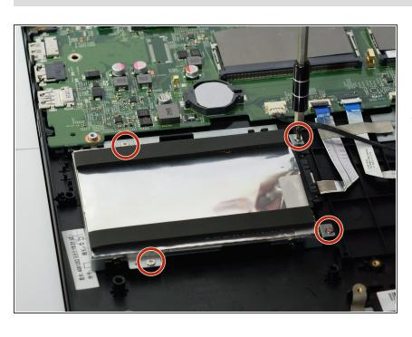
With the Phillips #0 screwdriver, remove the 4 M2 x 4.0mm screws holding the HDD case to the laptop body.
