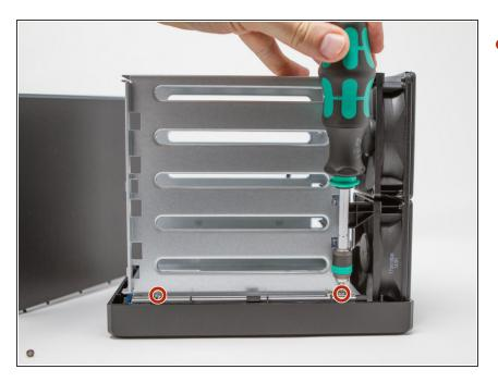
Then 2 screws on the upper face of the device (top).
