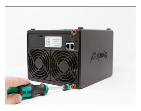
Remove the 2 screws on the back of the case at the top and bottom (not the one above the USB port)
