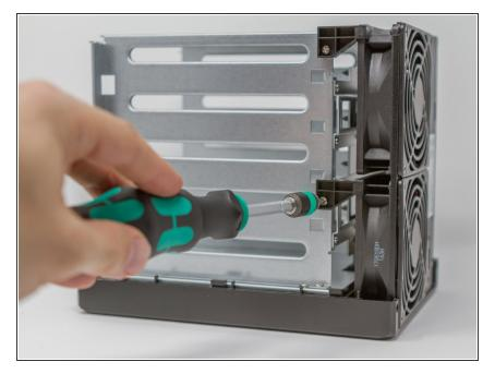
Remove the screws from the two shims to secure the disc cage and the two fans.
