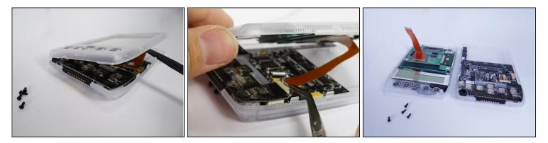
• Disconnect the flex strip from the motherboard with <u>tweezers</u>.
