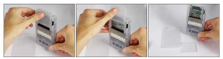
• Slide the memory cartridge cover up and off the device.
