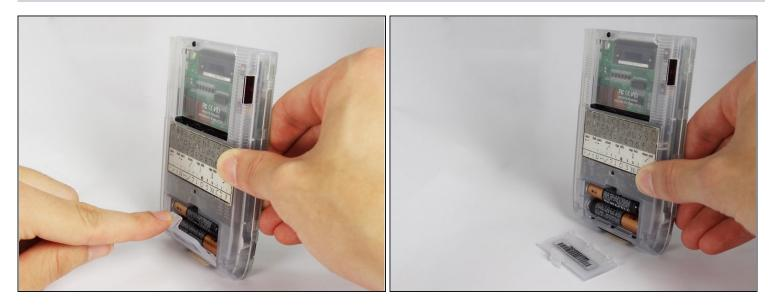
• Remove the battery cover by releasing the clip from the main body of the device.
