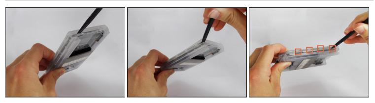
• Use the spudger to pry open the casing by applying pressure at 4 clips on both sides of the device.
