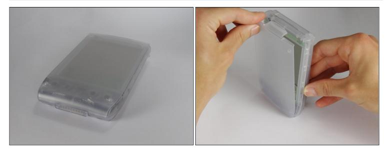
• Remove the outer screen cover by releasing the top clip from the main body of the device.
