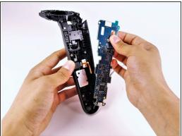
Lift the motherboard up and out of the Vive controller using your hands.
