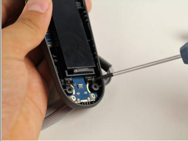
• Use the T5 Torx screwdriver to remove the two silver 4.2mm screws from the bottom of the battery frame.
