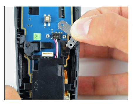
Remove the silver plate by pinching it with two fingers and lifting up.
