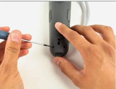
Use the T5 Torx screwdriver to remove the two black 5.2mm screws on the back gray panel.
