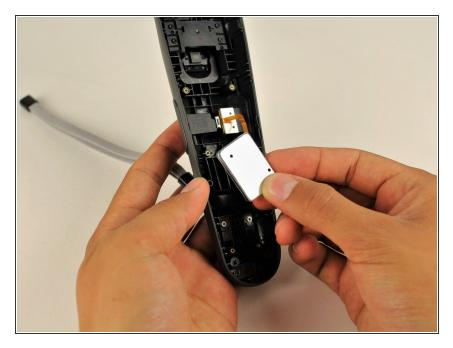
Lift the silver rectangular plate up and out of the controller using your hand.
