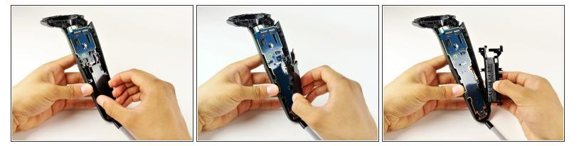
Lift the battery frame to remove the battery from the Vive controller
