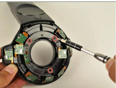
Use the Phillips 00 screwdriver to remove the three silver 12.8mm screws from the exposed upper sensor panel.
