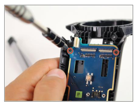
Use the Phillips 00 screwdriver to remove the two black 5.8mm screws from the top of the motherboard.
