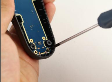
Use the T5 Torx screwdriver to remove the two silver 4.2mm screws from the bottom of the motherboard.
