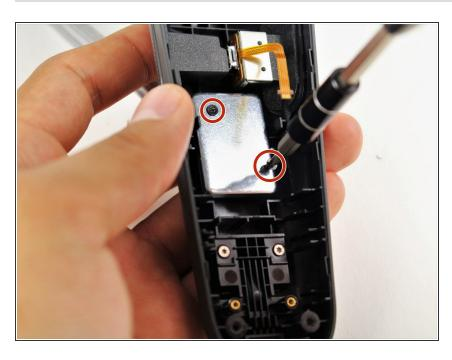
Use the Phillips 00 screwdriver to remove the two black 5.8mm screws from the silver rectangular plate.
