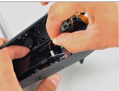
Disconnect the middle ribbon cable gently by pulling the ribbon cable up and away from the motherboard with two fingers.
