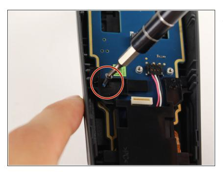
Use the Phillips 00 screwdriver to remove the black 5.8mm screw from the top left of the battery frame.
