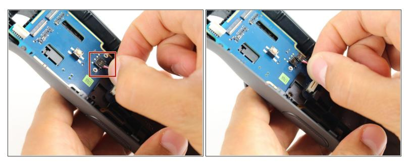
• Disconnect the three-pin cable gently by pinching the cable with two fingers and pulling up.
