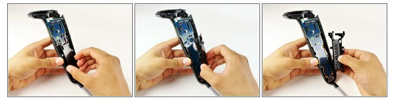
Lift the battery frame to remove the battery from the Vive controller
