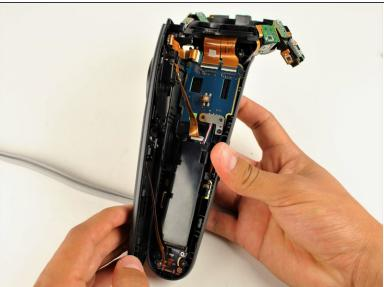
Use the nylon spudger to separate the front panel gently by running the spudger around the edges
