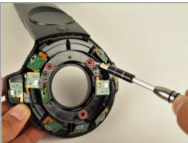
Use the Phillips 00 screwdriver to remove the three silver 12.8mm screws from the exposed upper sensor panel.
