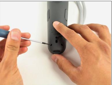
Use the T5 Torx screwdriver to remove the two black 5.2mm screws on the back gray panel.
