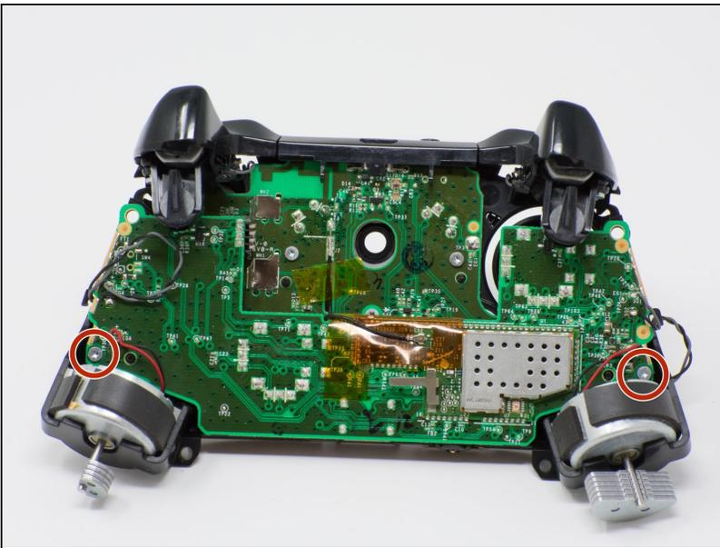
⚠ If the rumble motors fall out of frame, the wires may disconnect from the motherboard. The wires will have to be soldered to reattach the motor.
