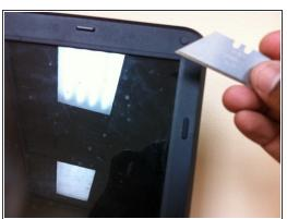
• First remove the stickers covers the screws in the 4 corners of LCD case. Stickers are very thin and using utility knife is easiest way to remove without damaging them. After removing stickers unscrew top 2 screws then proceed to Step 2 before trying to remove bottom 2 screws.
