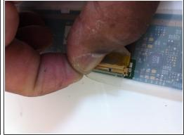
Before trying to remove video cable from back of LCD. First gently remove cable from adhesive holding it down to board. Then remove tape from top of cable holding connector in place. Be very gentle at these points.
