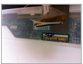
Now gently pull tab to pull cable from slot, be careful not to pull too hard and damage pins when removing. Once removed remove board and install new one.
