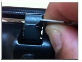
Turn laptop around to back, and undo the 2 latches in back in order to remove bottom 2 screws of LCD screen. Use your utility knife to slide into crack and push down to unlatch.
