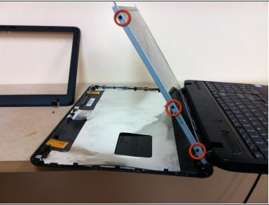
• Remove 2 screws at bottom of LCD frame and also the 2 screws at top of LCD frame (not pictured). This will allow you to lay the back cover away from frame to access side easier and remove the 3 screws on each side to detach LCD screen. Do not pull LCD once unscrewed, lay down face down on keyboard for last step.
