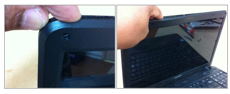
Once screws are removed, remove cover bezel from LCD very gently without breaking it, you should hear clicking noise when removing.
