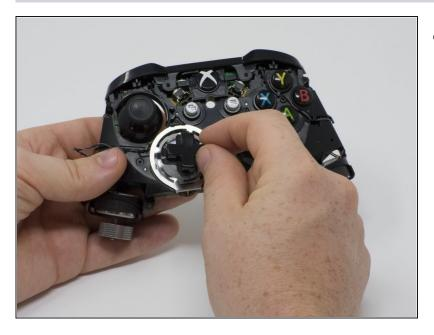
Turn the device over and remove the directional pad by gently pulling it away from the controller.
