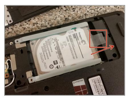
With the laptop's battery side facing you, pull the hard drive caddy's tab to the right.
