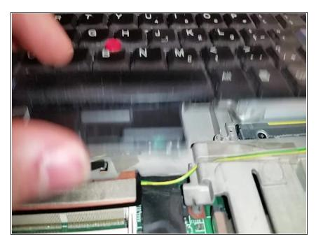
Pull up on the two little tabs jutting towards the screen to pull the keyboard connector off of the motherboard.
