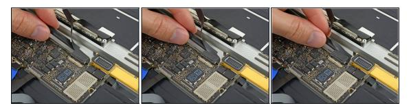
• Carefully slide the flat end of a spudger underneath the display cable to separate the adhesive holding it to the lower case.
