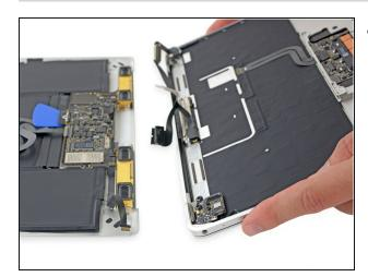
Separate the upper case assembly from the lower case assembly.
