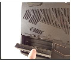
• Lift the battery while unlocking the lock circled in red.
