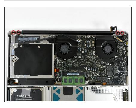
Remove the two outer 6 mm Torx screws securing each side of the display to the upper case (four screws total).
