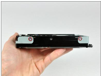
• Remove the two T10 Torx screws from both sides of the hard drive (four screws total).
