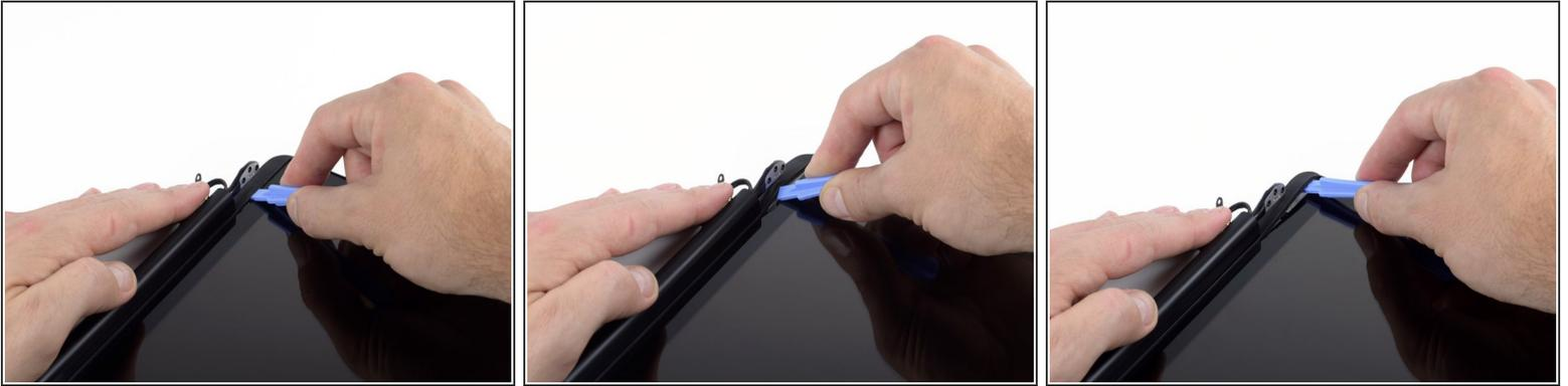
**i** It's very easy for the rubber display gasket to deform when exposed to heat, so it is best to remove it before using a heat gun to remove the display glass.
