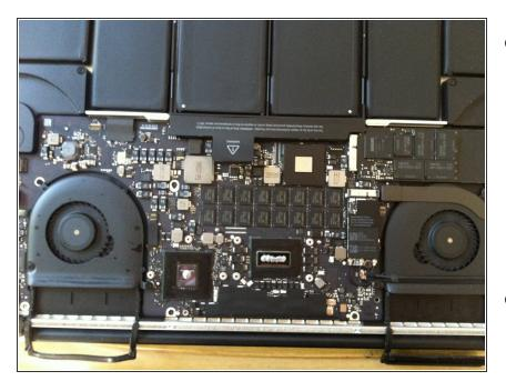
Re-apply your quality thermal paste to the now shiny clean CPU and GPU. DO NOT use too much. We don't want to overdo it like Apple. A line the size of a grain of rice on both the CPU and GPU should be perfect. \*\*You do not need to apply thermal paste on the heatsink as well - only on the CPU and GPU.
