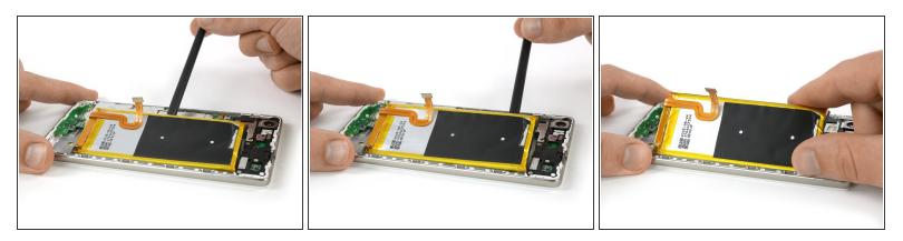
• Undo the adhesive beneath the battery with the Spudger.
