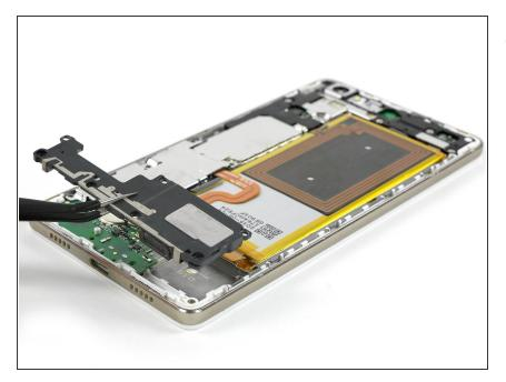
• Remove the loudspeaker carefully.
