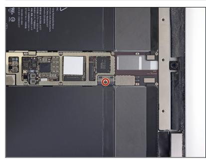
• Use a Phillips screwdriver to remove the 1.8 mm screw securing the battery connector.
