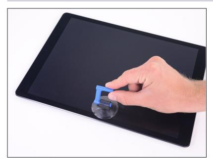
• Attach a suction cup to the left edge of the iPad's screen, above the Smart Connector port.
