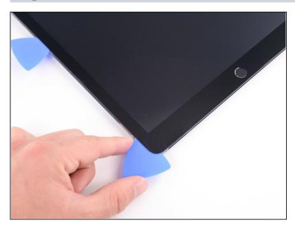
• Insert a pick in the bottom left corner of the iPad to prevent the adhesive from resealing.
