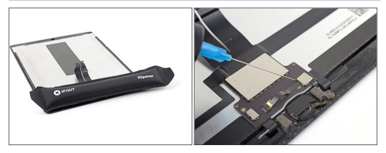
The home button's ribbon cable is **very** fragile. If it gets damaged, Touch ID will no longer function.
