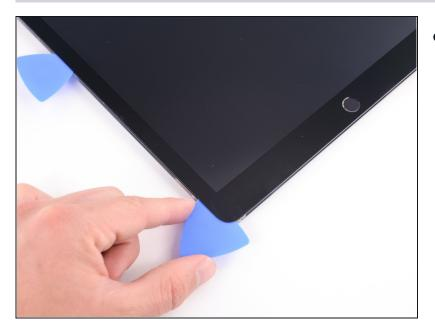
At this point, you've sliced through most of the screen adhesive. Use an opening pick to carefully slice any remaining adhesive along the edges until the screen is freed. If some parts are stubborn, heat the area with an iOpener to loosen the adhesive.
