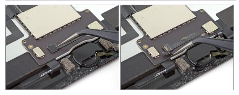
• Use tweezers to remove the tape covering the ZIF connector above the home button.
