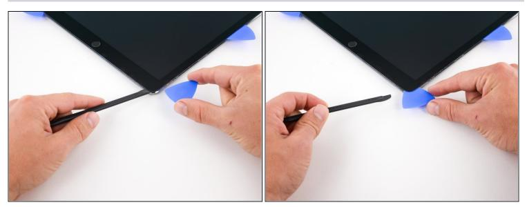
• Leave an opening pick in the lower right corner of the iPad to prevent the adhesive from resealing.
