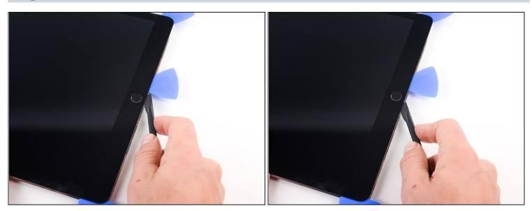
• Slide the tip of an opening pick or a halberd spudger to cut the adhesive below the home button.
