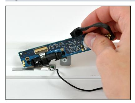
Lift the camera board out from the front bezel.
