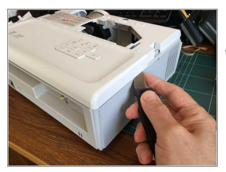
Release the top cover by running a spudger around all 4 sides. Remove the cover.
