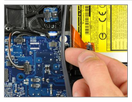
Move the SATA data cable away from the edge of the optical drive.
