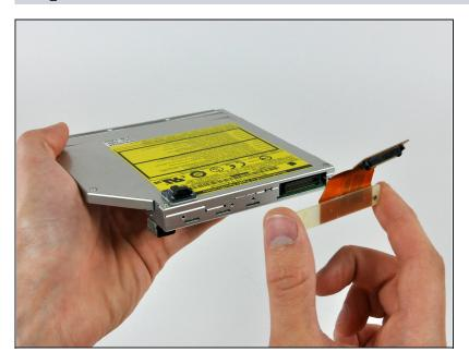
Pull the optical drive flex cable connector away from the optical drive.
