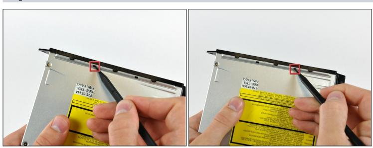
• Push the two optical drive bracket tabs out of their slots in the top of the optical drive.
