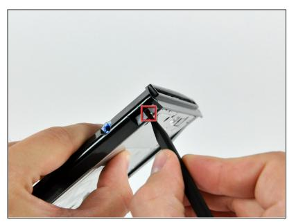
Using the tip of a spudger, press the optical drive bracket tab out of its slot on the side of the optical drive.
