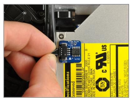
• Disconnect the optical drive thermal sensor.
