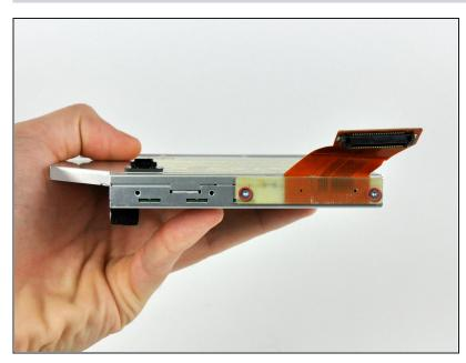
Remove the two T6 Torx screws securing the optical drive flex cable to the optical drive.
