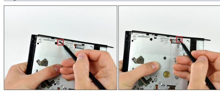
• Use the tip of a spudger to push the optical drive bracket tabs out of their slots on the bottom of the optical drive.
