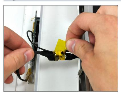
If necessary, remove the piece of kapton tape wrapped around the microphone and camera cables.
