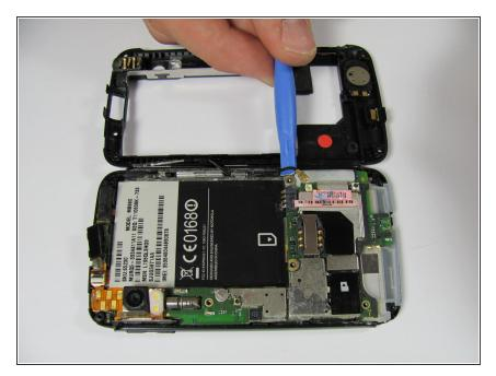
• Disconnect the antenna from its housing on the motherboard by gently lifting beneath it.
