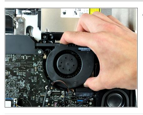
Lift the optical drive fan off the plastic posts protruding from the rear case, minding any cables that may get caught.
