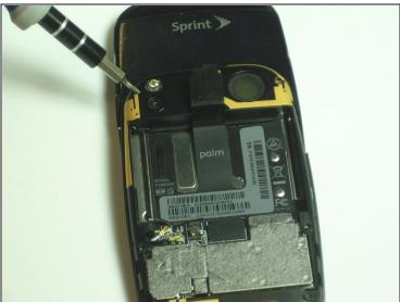
• Use the T5 Torx Screwdriver to remove the six screws holding the backing frame in place.
