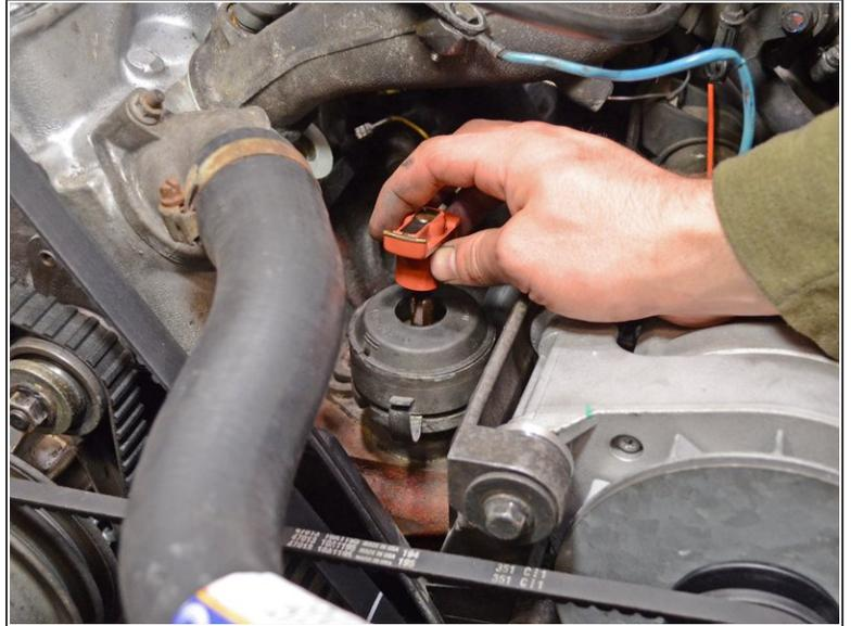
**i** The distributor rotor sits directly underneath the distributor cap and is not held in place by any screws or fasteners.
