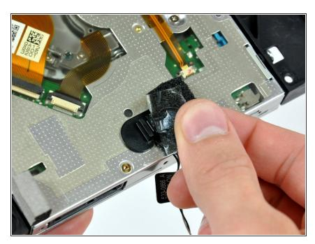
Remove the piece of foam tape covering the optical drive thermal sensor.
