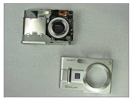
Separate the front case from the body of the camera.
