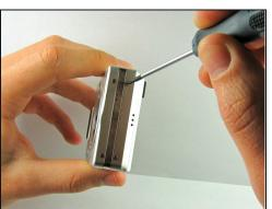
Remove eight 1.8 mm screws from the left and right sides of the camera using a Phillips #00 screwdriver
