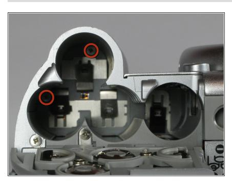
Remove the two 4.1mm screws at the bottom of the battery flap.
