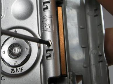
• Remove the 2.4mm screw located underneath the cover of the memory card slot.
