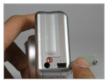
Remove the 3.8mm screw underneath the flap that covers the A/V port.
