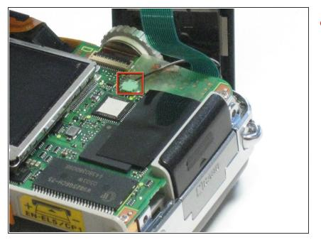
Disconnect the cable by pulling the head upward along the green circuit board. If you only are changing the LCD, skip this step.
