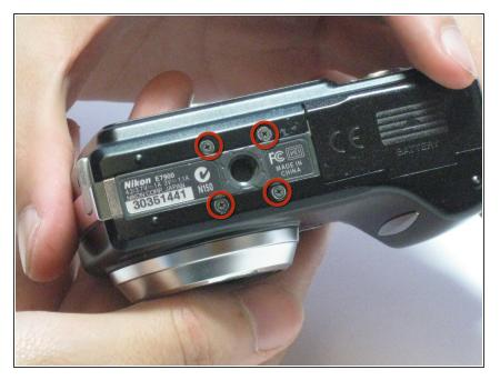
• Remove the four 3.0mm screws on the bottom of the camera.
