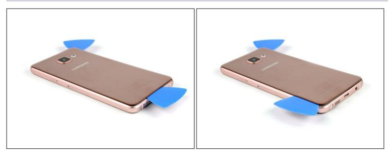
• Insert a second opening pick and move around the other corner at the bottom part of the back cover.
