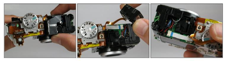
• Gently wiggle the eyepiece out of its place. It should snap out of place.
