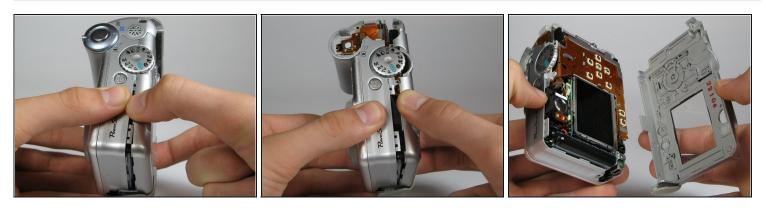
• Separate the back casing and front casing of the camera using your hands.
