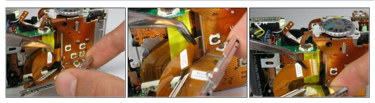
• Gently grasp and pull the cable from the motherboard. The cable should easily slide out.
