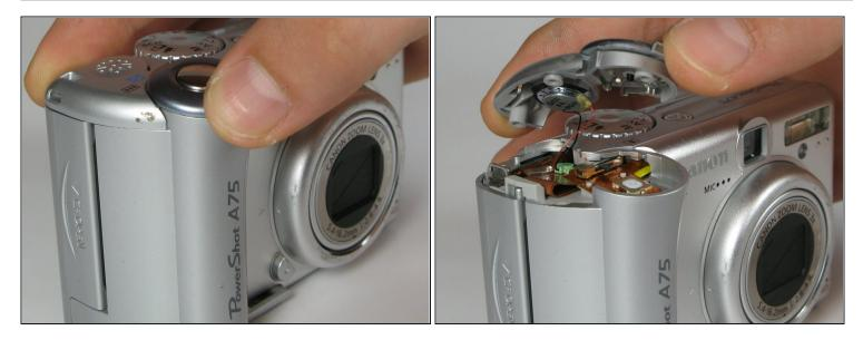
Lift the shutter button and speaker part from the top of the camera.
