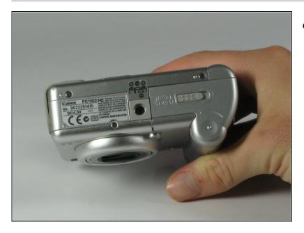
• Turn the camera over and locate the "BATT OPEN" sliding switch.
