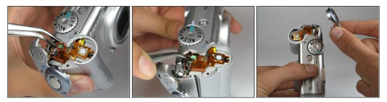
• Using a pair of <u>tweezers</u>, grab the plug that connects the speaker to the camera and gently pull it out.
