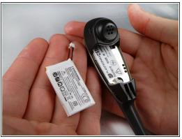
Locate and detatch the white connector that connects the wires of the battery to the wires of the headset.
