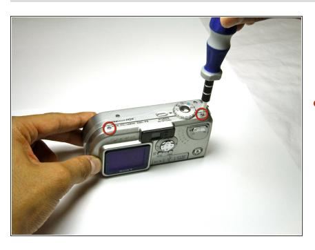
Unscrew the four 3.0mm Phillips #000 screws holding the back case onto the camera; there are two
