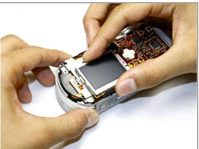
Unlatch the display by sliding it towards the circuit board.
