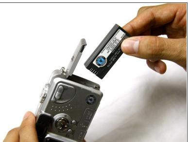
Remove the battery from the camera.
