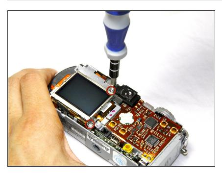
Remove the two 3.0mm Phillips #000 screws holding the display to the metal backing.
